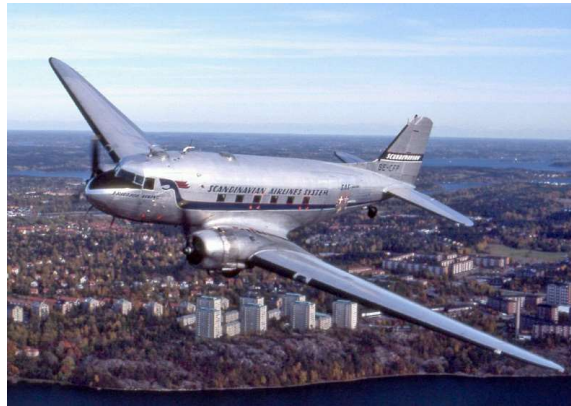
DC3 (1936) requirements: Wright Flyer reqs. + Passengers and cargo + 1000mi range + Basic reliability
